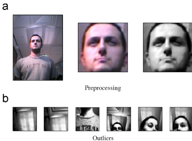
Fig. 8. Data preprocessing: (a) Left to right—typical input frame from a video sequence of a person performing unconstrained head motion ( 320 \times 240 pixels), output of the face detector ( 72 \times 72 pixels) and the final image after resizing to uniform scale ( 50 \times 50 pixels) and histogram equalization. (b) Typical outliers—face detector false positives—present in our data.
