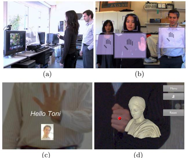
**Figure 1: Gesture interface.** (a) set up of camera mounted on top of the screen and multiple users in the field of view, (b) interaction is initiated by hand detection, (c) face detection is performed during the attention phase, (d) a sample application for the inspection of 3D models.
