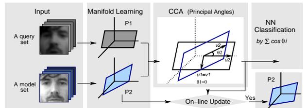
**Figure 4: Face recognition by matching image sets.** The similarity between manifolds is computed as the sum of principal angles and is used for NN classification. Once a query set has been classified, it can be included in the model by on-line updating the existing manifold.
