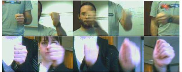
**Figure 2: Appearance variation of hand regions.** *Shown are cropped hand regions from test sequences. Motion blur, changing pose and other skin coloured objects make tracking challenging.*
