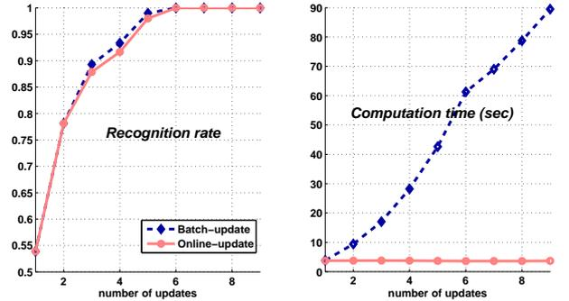
**Figure 8: Face recognition results.** (left) Accuracy improvement of the on-line and batch-method for the number of updates. (right) Computational time of the two methods.
