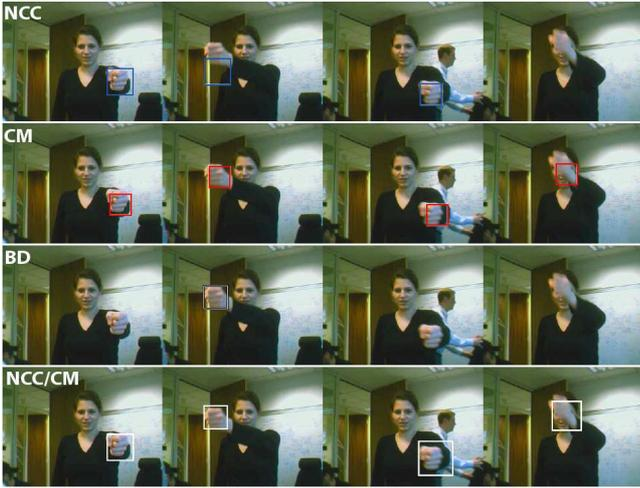
**Figure 6: Comparison of individual trackers with combined NCC/CM tracker.** This figure shows snapshots of a sequence and results of the NCC tracker, the CM tracker, frame-by-frame detection and the proposed NCC/CM tracker.
