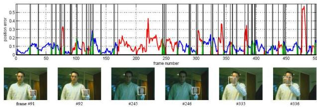
**Figure 9: Switching trackers over time.** This figure shows the tracker’s switching behaviour, colours in the plot indicate the component at each frame (blue=NCC, red=CM, green=detector). During this sequence the light was turned off and on. Example frames where transitions occur are shown below (first and third pair from NCC to CM due to motion blur, middle pair from CM to NCC via local detection).
